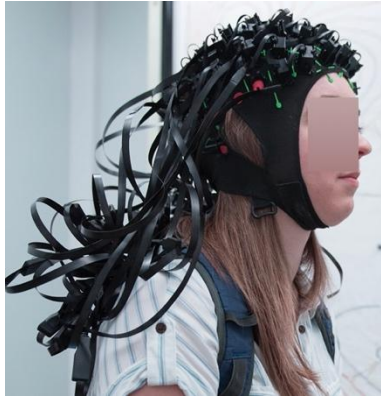
Figure 2: Example of a 50-channel OPM system (Figure courtesy of Matt Brookes).
