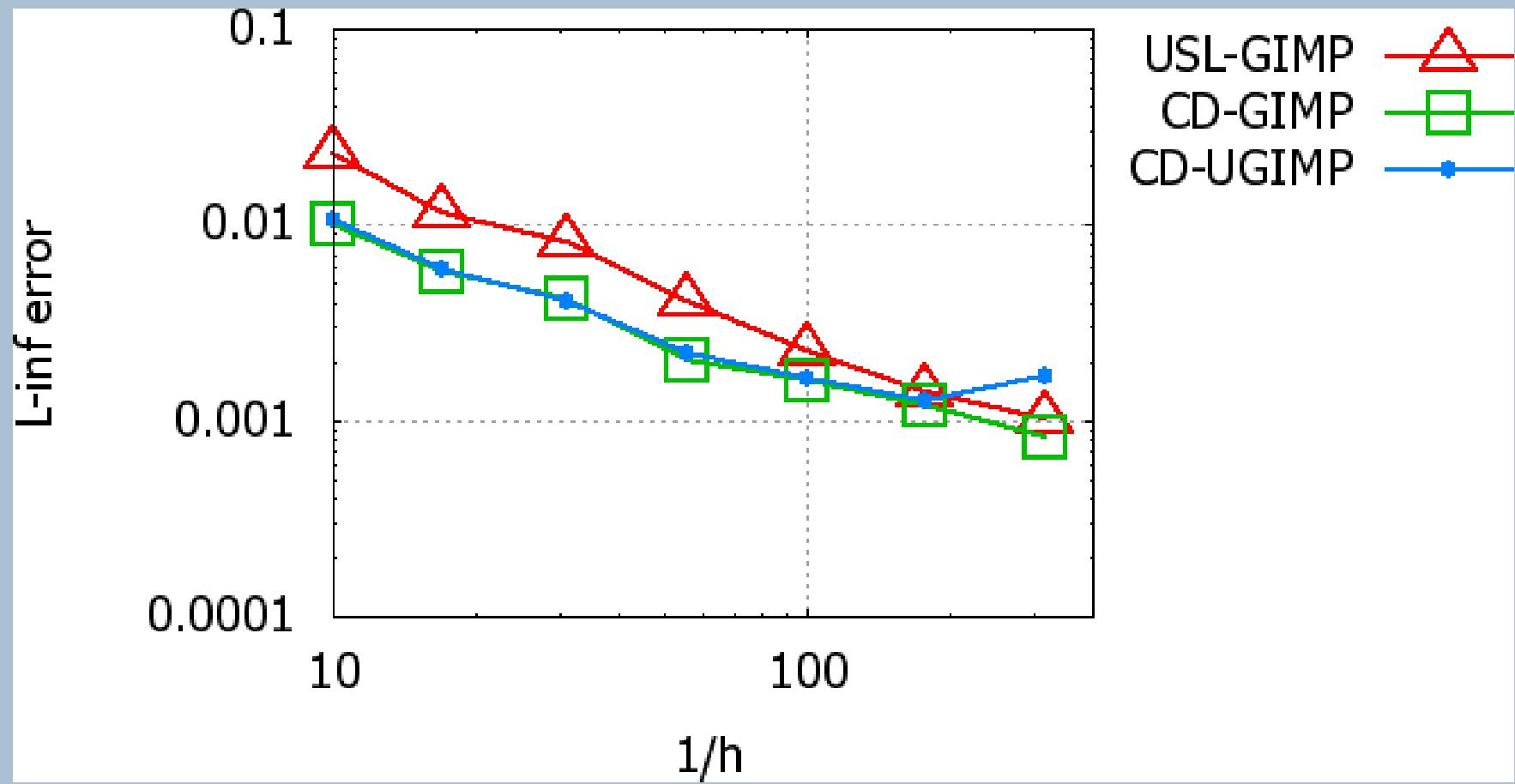
The miss-alignment of particles and the stair-stepped surface now dominate the error.
