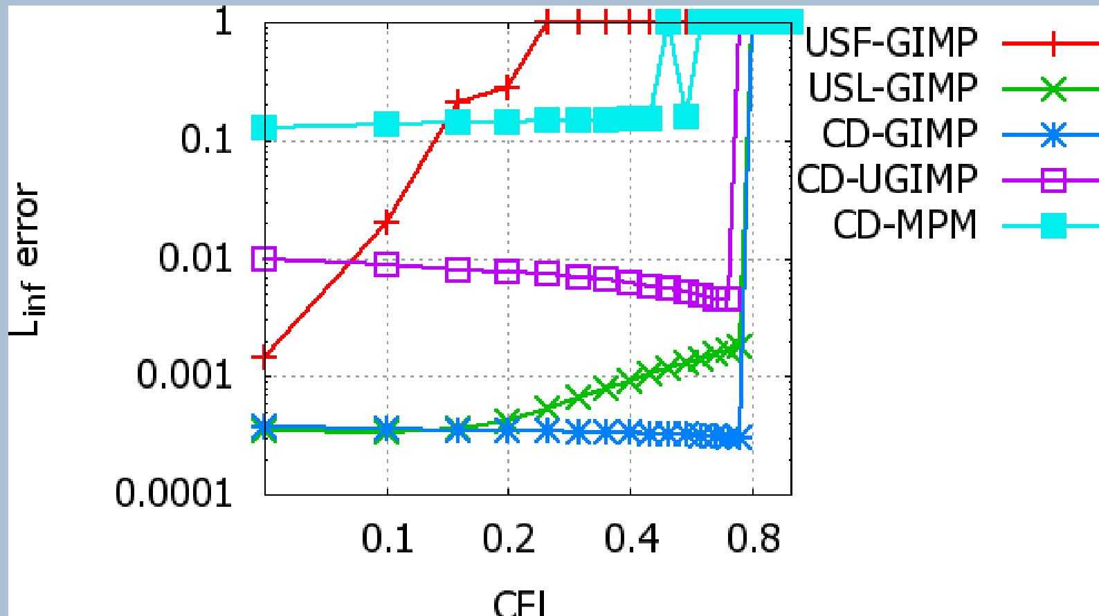
Most methods display zero temporal convergence until stability is lost, even though CD-GIMP is formally 2<sup>nd</sup> order in time.
