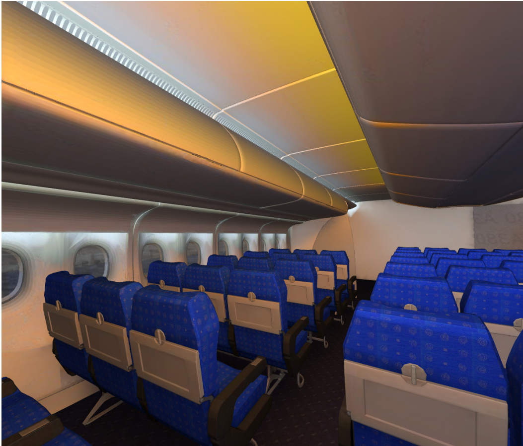
Figure 5: Low resolution geometric model with results from high-quality lighting simulation. More than 600 MB of texture memory are required to visualize these results interactively.
