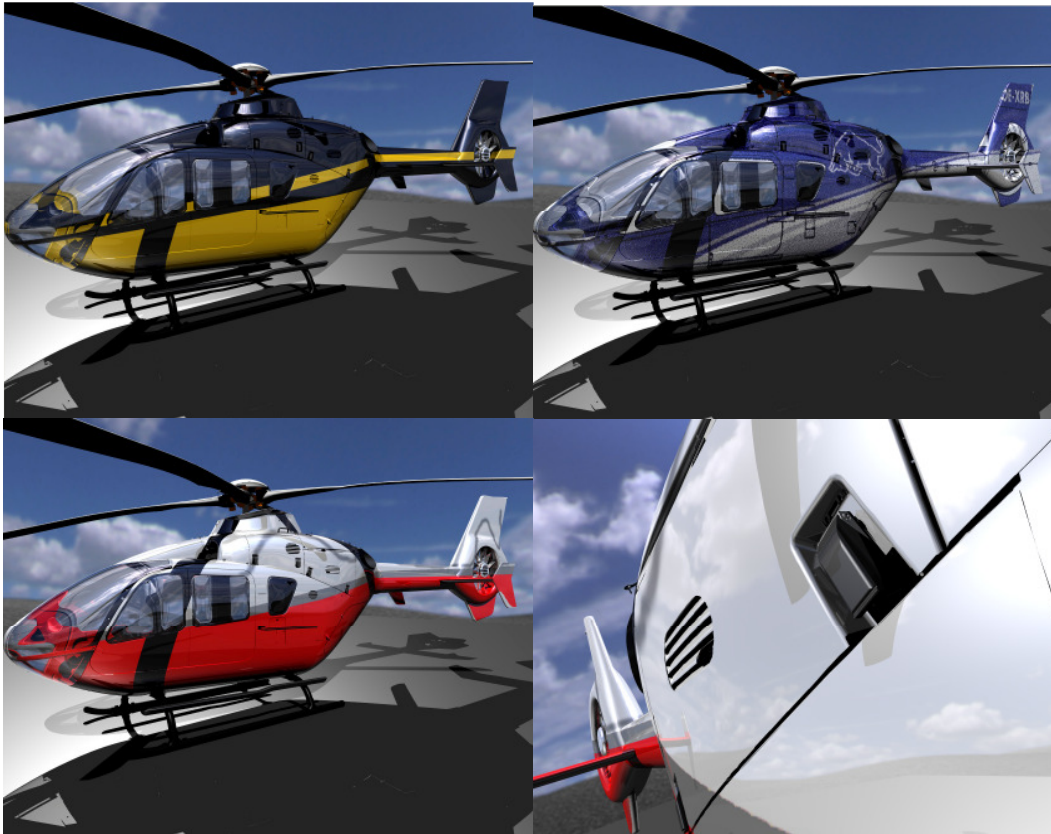
Figure 6: Different paint design for a helicopter visualized interactively with real-time ray tracing. The highly specular material results in significant reflections that need to be taken into account during the design. The close up shows the physically accurate reflection evens on curved surfaces.
