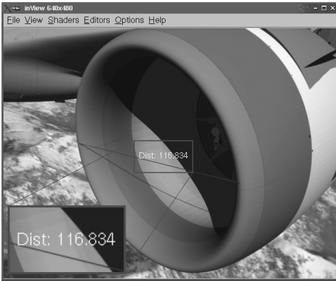
Figure 2: 3D CAD review features: (a) Measuring the diameter of a Boeing 777 engine. (b) All components can be pixel-accurately identified by simply moving the mouse pointer over them.
