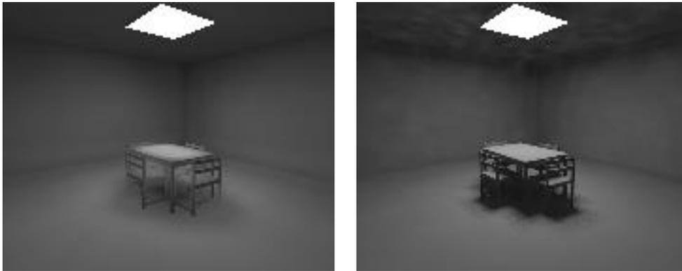
Figure 4.4: Improvements due to independent calculation of direct light. Note the sharper shadows in the right image, especially on the chairs.
