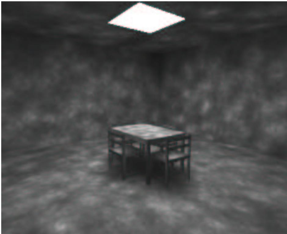
Since lower frequencies are easier perceivable to the eye than higher frequencies, this kind of noise is especially perceivable. Increasing  $k$  decreases the frequency of the noise, blurring it, but not removing it. The noise in the estimate can also be reduced by increasing the photon density, which will also increase rendering time and memory requirements (see section 3.1). Using a local pass completely remove low-frequency noise from diffuse illumination, but also increases
