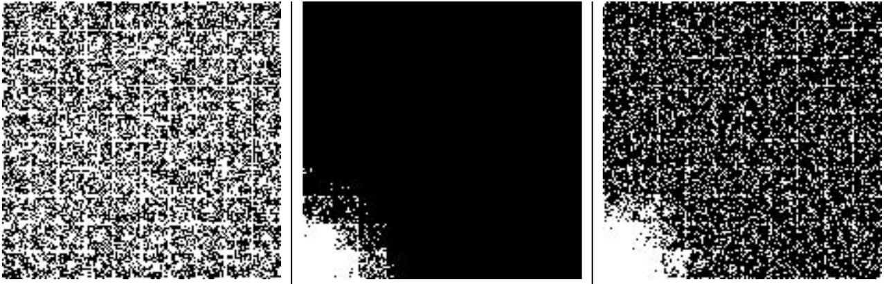
Figure 4.12: Using importance in generating the photon map: The left image shows the position of the photons in SCENE10 (10 by 10 rooms, viewed from the top) as generated with the original random walk without using importance. The center image depicts the locations of the importons, while the importance-driven map generated by this importance map is shown on the right.
