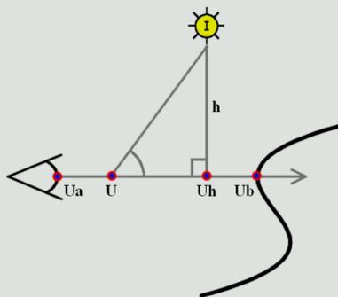
Figure 1: Illustration of the terms involved in the computation of the air-light integral.
