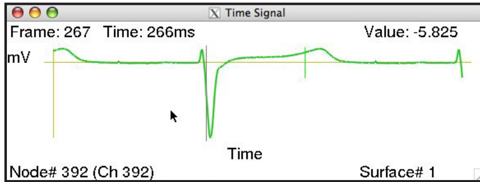
Figure 2: Time signal window layout. Vertical line indicates the frame currently displayed in the surface plot. Text annotations can vary with the data content and mode settings.
