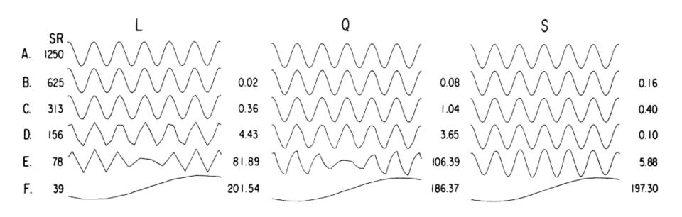
35 Hz sine wave Linear, quadratic, sine x/x reconstruction
