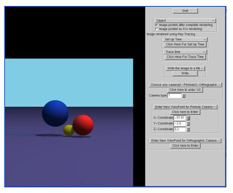
I have extended my integrated viewer by allowing the users to change the viewpoint interactively through entering the new point or clicking on the spinner object. I have also allowed the user to switch between the orthogonal camera and pinhole camera.
