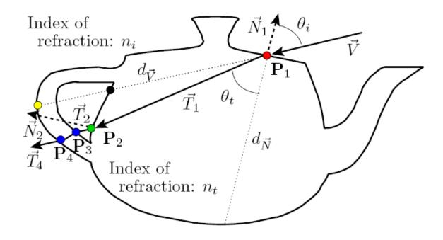
Here an approximated approach is used to calculate refraction through two interfaces with values easily computable via rasterization. The method proposed uses two passes to compute the doubly refraction.
