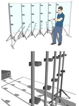
Fig. 1. Concept picowall module consisting of 18 projectors, driven by a single workstation with 6 outputs and six 3-way splitters. Projectors are mounted with lightweight, inexpensive photography equipment, designed for easy micro-adjustment.
