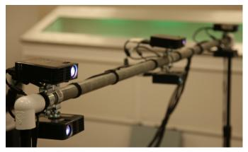
Fig. 2. Projector mount. We secure six projectors horizontally onto a single  $6' \times 1.5''$  steel pipe, and use stainless steel brackets for individual mounts. Using microphone stands, the resulting construction is stiff. A similar outcome could be achieved with a sufficiently rigid photography backdrop kit.
