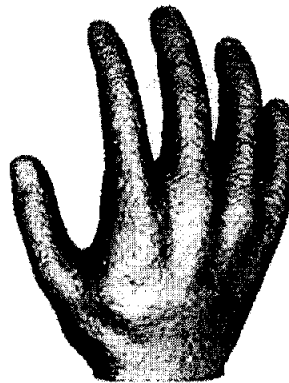
Figure 10. To demonstrate robustness in the presence of noise, we added Gaussian noise to laser range scanner data. The resulting model is still watertight.
