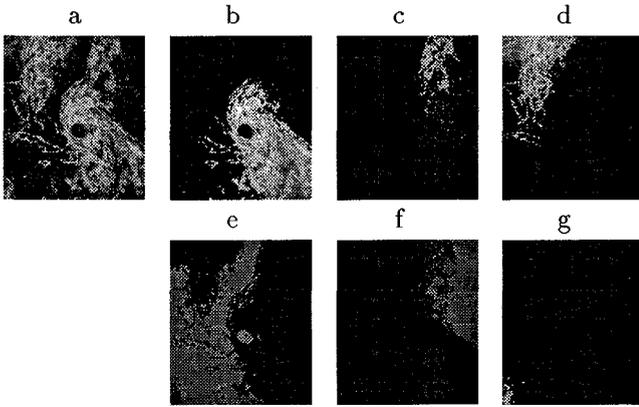
Figure 6: (a) shows a 126x106 weather radar image. (b)-(g) show the components of the partition with  $N_{cut}$  value less than 0.08. Parameter setting:  $\sigma_I = 0.005$ ,  $\sigma_x = 15.0$ ,  $r = 10$
