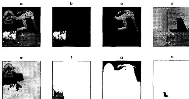
Figure 5: (a) shows a 80x100 baseball scene, image intensity is normalized to lie within 0 and 1. (b)-(h) shows the components of the partition with  $Ncut$  value less than 0.04. Parameter setting:  $\sigma_I = 0.01, \sigma_X = 4.0, r = 5$ .
