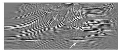
larger. Seismic interpreters look for these "bright spots" to find oil and gas. The layers above also are bright, but their brightness does not vary as strongly across the layers. Many seismic reconstruction algorithms have difficulty imaging this target because of the faults above it.
