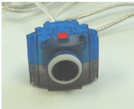
Figure 4 Lego camera used temporarily to record UBROBO activities from the robot's view
