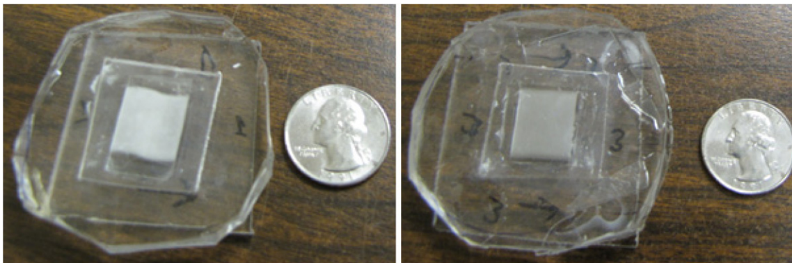
Figure 13. The pictures of two assembled MRI phantoms (left: with curved channels, right: with straight channels) along with a US quarter coin. Each phantom is placed in a square water reservoir formed by the PDMS cap and PDMS substrate. No air bubble can be seen in the phantom assembly.
