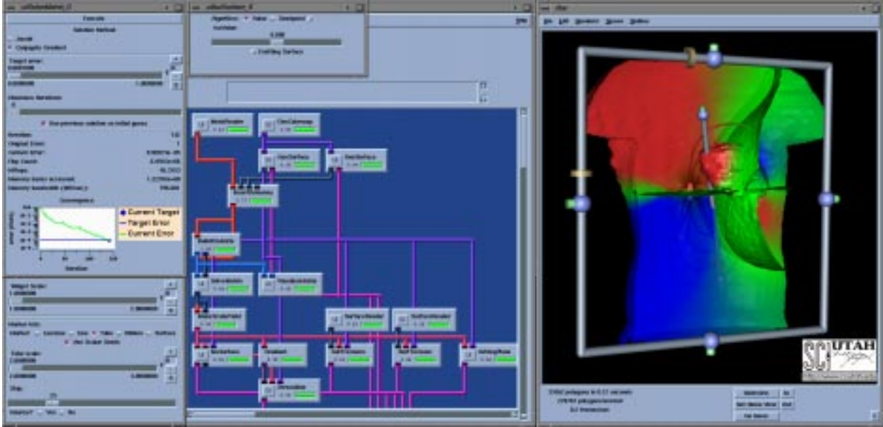
Figure 1: An example SCIRun network, showing the dataflow programming interface, user interfaces for controlling simulation parameters, and results from an large finite element model.
