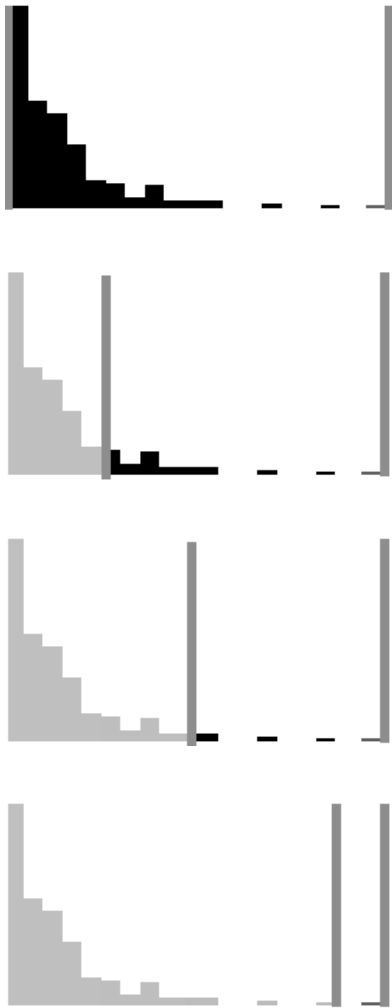
Figure 3. This series shows a simplified version of the histogram in order to demonstrate how the visualization technique proceeds. It begins with all mesh elements, as displayed in Figure 2. The lefthand range bar is moved right in a series of steps. Only those mesh elements within the two range indicators are drawn.
