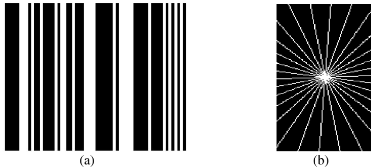
Fig. 1. (a) Image showing the binary mask for a single image direction to undersample full k-space data in variable density fashion by a factor of two. Six lines around the center of k-space are sampled and the lines outside are sampled in a random fashion. The white portion represents the region of k-space sampled. The phase encoding direction is horizontal. (b) Image showing the binary mask for a single image direction to undersample full data in radial fashion. White portion is the region of k-space sampled.
