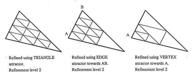
Graded meshes can be obtained in the following way. Consider a triangle to be refined with a TRIANGLE attractor. Then all its neighbouring triangles which share an edge with it, are refined towards that shared edge. Similarly, all triangles with a vertex in common with the original triangle are refined towards that vertex. Finally
