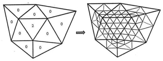
where dashed lines represent the bisecting edges of green triangles. The concept of IFS attractors thus provides an elegant way to implement multiple levels of regular refinement.
