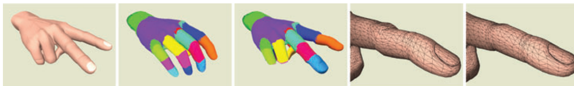
Figure 2: Motion decomposition together with fuzzy kd-trees allow for ray tracing deforming meshes by decomposing the motion of the mesh into an affine transformation plus some residual motion: (a) one frame of an animated hand; (b) the deforming mesh is split into sub-meshes of similar motion, shown in the rest pose; (c) reconstruction of frame (a) using the affine transformations of each cluster only; (d) close-up view of (c) revealing the erroneous mesh when approximated only by affine transformations; (e) adding the residual motion handled by the fuzzy kd-trees yields the original mesh.
