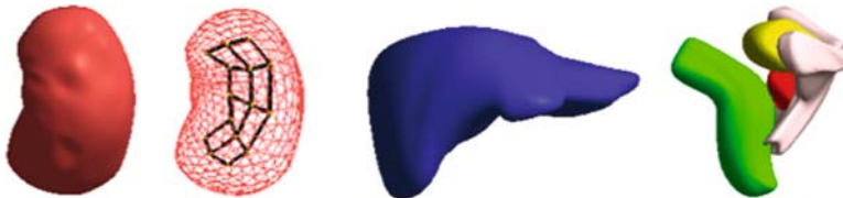
Fig. 9.2 M-rep modeled kidney with its medial mesh, a liver model that is made from two figures, one for each lobe, and male pelvis model made from multiple objects (two bones, bladder, rectum, prostate). The kidney model also shows the underlying representation of a sampled medial surface and a tiled boundary
