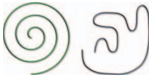
Fig. 2. Both of these curves exhibit very similar curvature magnitude values. Therefore, a single global measure fails to distinguish streamlines sufficiently. In this case, the tortuosity attribute would fair better but there are cases where this would also fail. A better method creates a distinctive signature for the streamlines using density-based attributes.
