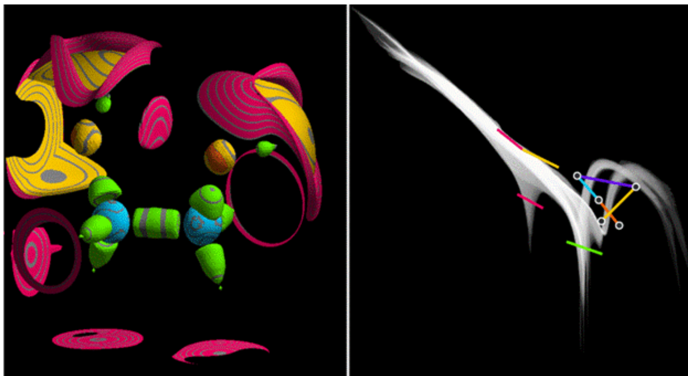
Figure 3.1.2b Interactive extraction of fiber surfaces from bivariate fields [36]. Right: Continuous scatterplots with colored selection of the fiber surface control polygon; Left: resulting colored fiber surfaces.
