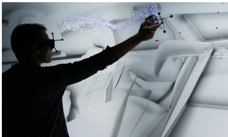
Figure 3.3.3a An engineer interactively exploring complex airflow inside an electric vehicle cabin by directly seeding particles in the flow. Credit: John De La Rosa, National Renewable Energy Laboratory.
