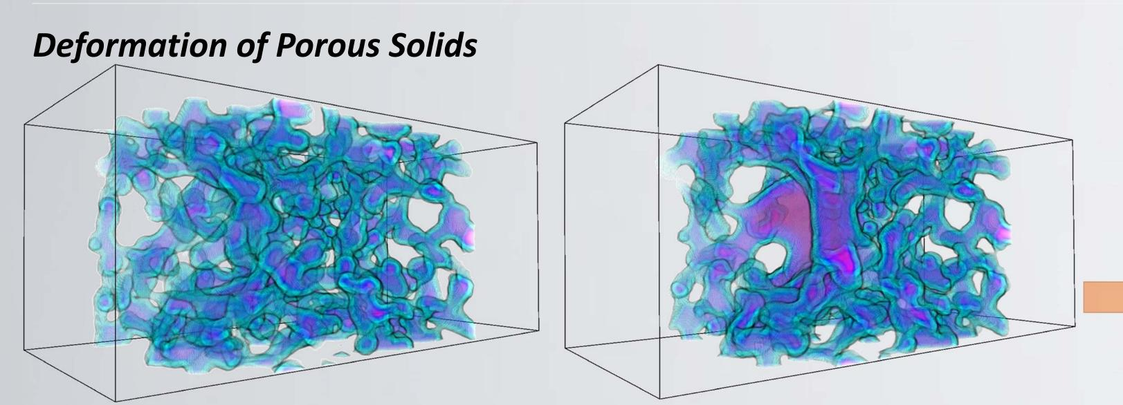
How an aerogel deforms is crucial in investigating its usability for spacecraft insulation. When a copper foam is struck by a micrometeoroid, a scientist wants to measure the loss in porosity and structural integrity of the material.
