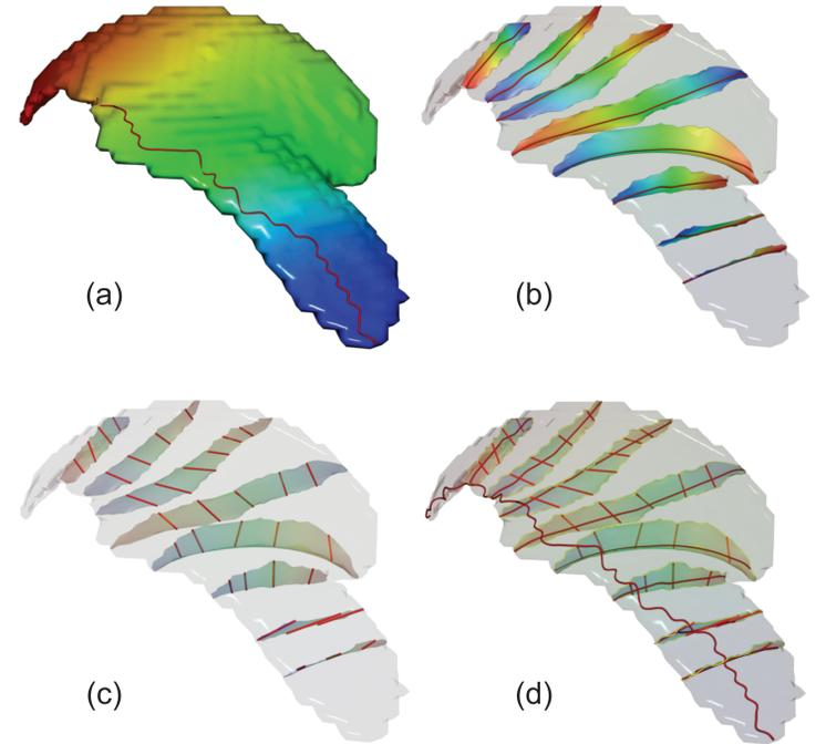
One of the primary drivers of auto-ignition and extinction is the rate of turbulent mixing, characterized locally by the scalar dissipation rate. Compressive strain in directions aligned to scalar gradients, creates thin pancake-like regions (shown above as (a)) in the simulation whose thickness provides a direct measure of the local mixing length-scale and its scaling with turbulence length scales.
