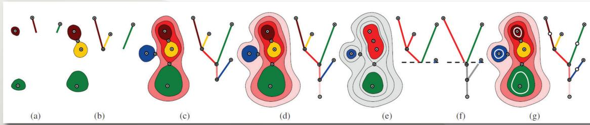
For the above figure, each color represents one "arc" or the merge tree. the image sequence (a-d) shows steps in a top-down construction of the tree. (e-f) shows how thresholds can be used to extract features from the tree, (g) shows relative thresholds.
