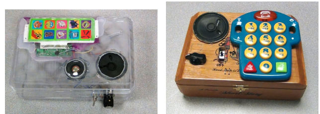
Figure 5: Noise-making toys modified by students through circuit bending / hardware hacking. The modified toys have been repackaged into new cases and new controls have been added.
