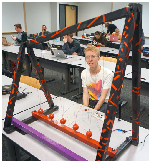
Figure 9: Final project of Jordan (chemistry major) in 2016. He constructed a set of pendulums that influence the sound of a multi-oscillator circuit by passing over light sensors in the sculpture’s base.
