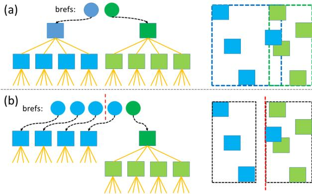
**Figure 3:** (a) A segment of two *BRefs*, corresponding to two object BVHs which overlap spatially. (b) The first *BRef* (dark-blue circle) is ‘opened’ and replaced with *BRefs* to its children, allowing the partitioning step to find a better partition with less spatial overlap.
