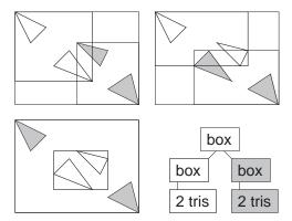
Figure 2: Different BVHs for 4 triangles. The siblings are allowed to spatially overlap (unlike spatial subdivision). Other possibilities include splitting to size 1 and 3 triangle list, and recursively splitting lists of 2 or 3 triangles.
