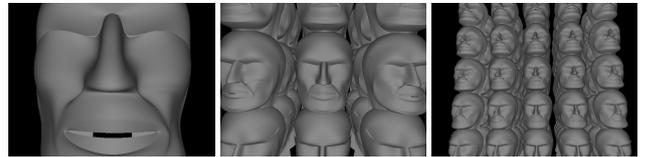
**Figure 5: The overall performance is largely independent of the actual number of patches and varies only by roughly 20% while zooming out from a single head model to a view where more than 125 head models are visible. Each head model consists of 915 subdivision patches and is rendered with four refinement steps at 1-2 fps on a single processor.**
