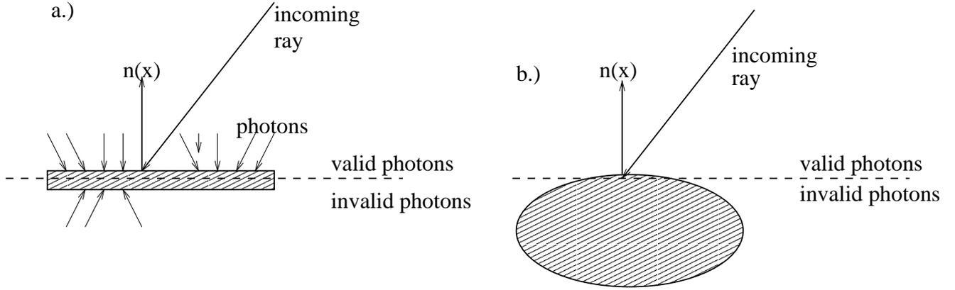
Figure 4.2: Specifying a culling plane by query position and surface normal (dashed line) yields another plausibility test. Considering photons 'behind' this culling plane invalid, illumination from the backside (as demonstrated in section 3.3.4) can be prevented on flat surfaces (as sketched in case a), but may be fatal on curved surfaces like in case b, where almost all photons on the ellipsoid are considered invalid.
