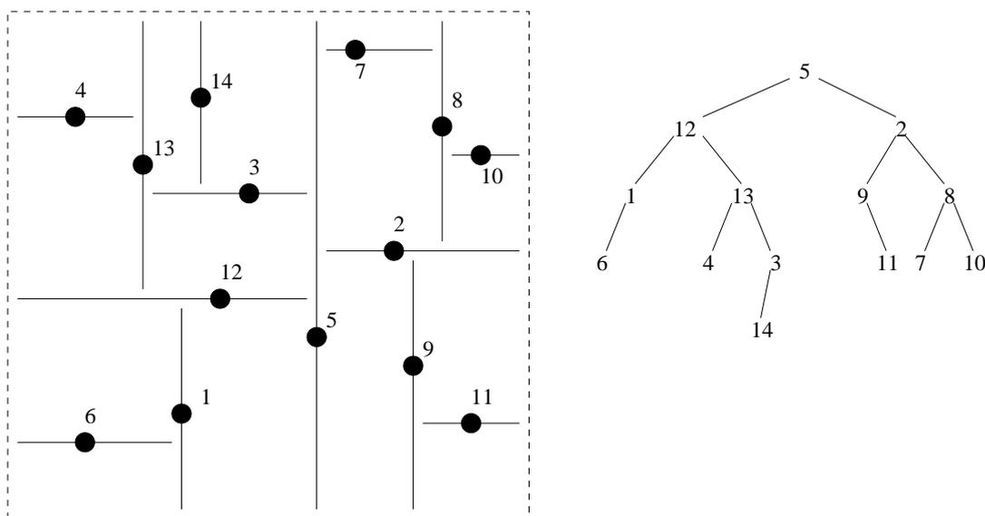
Figure 2.1: A sample kd-tree for  $k = 2$  (not balanced).
