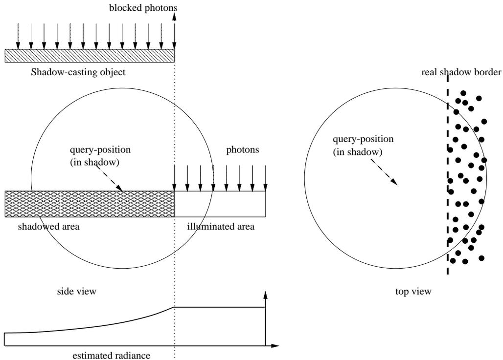
Figure 3.2: Blurring of shadow borders: The query ball is extended until it contains the required number of  $k$  photons, even if the query-position is in complete shadow.
