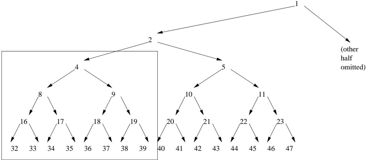
Figure 2.2: Non-sequential numbering of nodes in a subtree. The nodes in the subtree with root node 4 are 4, 8, 9, 16, 17, 18, 19, 32, ...
