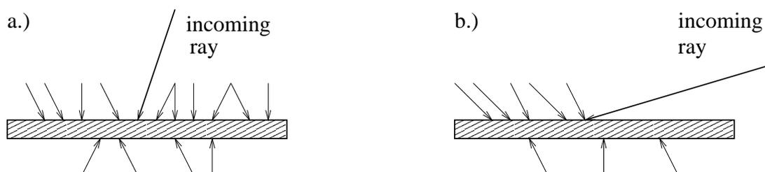
Figure 4.1: A simple plausibility test: Testing the angle  $\alpha = (\omega_{ray}, \omega_{photon})$  to be below 90 degrees is simple and seems promising in case a. However, it would be a bad classification in case b. Similar cases can be constructed for other tests.
