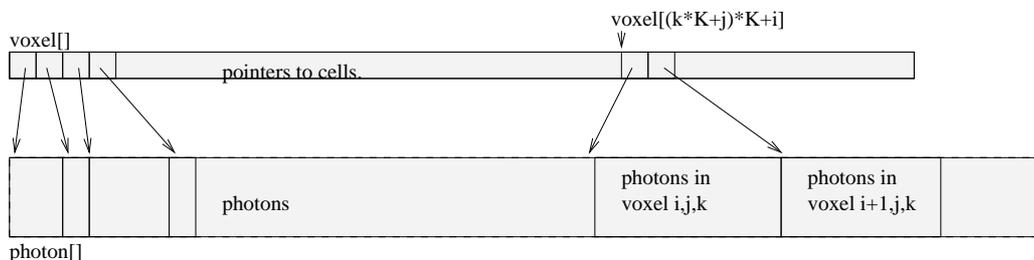
As compared to a kd-tree, the regular grid is not adaptive, and therefore reaches optimal performance only when photons are well distributed in the scene. While this is often the case for diffuse photons, it may be problematic with caustic photons, which tend to be clustered. Specifying a maximum search-radius yields performance-gains even in this case.
