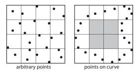
Figure 3: In scattered data most or all cells need to be refined, defeating the purpose. In a suface (curve in 2D) there are cells (shaded) that need not be refined.
