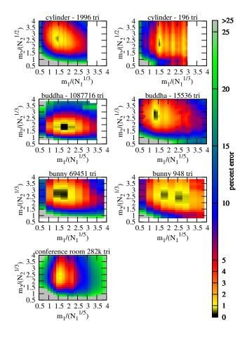
Figure 5: Percent error in rendering times found through an exhaustive search across the 2*D* parameter space for creating 2-level grids. Moving across the *x*-axis changes  $m_1$  and the *y*-axis corresponds to  $m_2$ . Our theory predicts the point (1.6,2) for the cylinders and (1.5,2) for the other models as being optimal.
