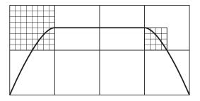
Figure 4: Two different ways to refine a cell.
