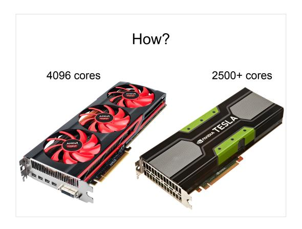
The primary mechanism by which such performance is possible is due to the ability of manufacturers to pack so many cores in such a small area. This leads to accelerator cards which can quite literally run thousands of 'threads' at once.
