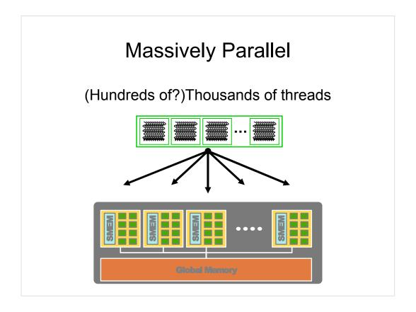
Of course, this processing power is only available if you know how to harness it. GPU processing requires developers to find parallelism at significantly finer scales than traditional techniques would require. Furthermore, programmers must be aware of architectural concerns, such as how threads may diverge and how to use memory efficiently, to get the peak performance from these processors.
