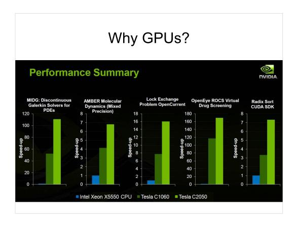
In recent years, the processing power of highly-SIMD RISC architectures, such as those employed by GPUs, has largely eclipsed conventional CPU performance.
