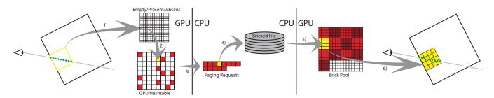
Figure 2: The missing brick reporting / paging subsystem of our volume rendering approach. Missing bricks are recorded into a hash table (1, 2), to be paged in (3, 4, 5) and rendered in subsequent frames (6).
