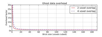
Figure 6: Brick size overhead. As bricks get smaller, the overhead for the additional ghost data grows significantly. At a larger brick size of  $128^3$ , the overhead with 2 ghost voxels per dimension amounts to a few percent, whereas with  $32^3$  bricks this increases the dataset size by almost 50%.
