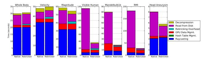
Figure 4: Time spent at various stages of our pipeline, aggregated over the generation of a rotation sequence. Comparisons are made between data stored with the ideal brick size for that dataset ('Native'), and data stored at a large brick size of 256<sup>3</sup> with the ideally-sized bricks created at run-time ('Rebricked'). 'Whole Body', 'Velocity', and 'Magnitude' suffer from a lack of ray saturation.
