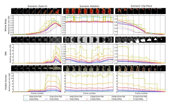
Figure 5: Working set sizes across three different scenarios for multiple datasets. Smaller brick sizes approximate the working set better.
