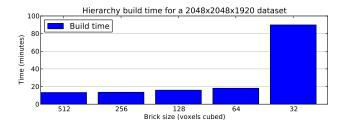
Figure 8: Time to build bricked representation for a medium-sized dataset, as a function of brick size. Renderers desire small bricks to perform efficiently, but generating such bricks takes significant preprocessing resources.
