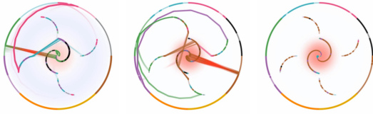
Figure 5.8. The material point method (MPM), a particle-based mechanical engineering simulation, in action. Left: Computation of momentum from the mass and velocity data (in the black and green arrays). The algorithm tends to sweep through the values in order, resulting in good cache performance. Middle: Computation of the particle stress update (brown data array) near the end of the timestep, from various data, including the constitutive model (blue data array). MPM is made up of several phases which tend to access the data in order. The resulting visual pattern is that of data moving into L1, being operated upon a limited number of times, and then slowly migrating first to L2 and then back into main memory, as newer data comes into L1 to be operated upon in turn. Right: This example shows a bigger MPM simulation and a larger cache to demonstrate the scalability of our visualization system.
