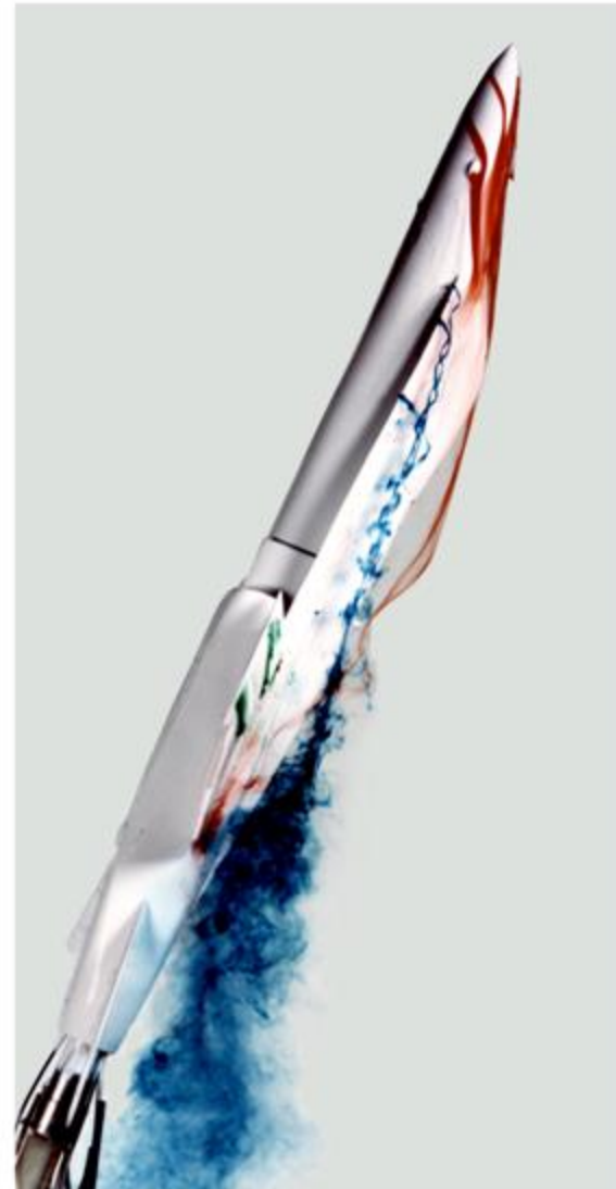
Dryden Flight Research Center ECN 33298-47 Photographed 1985 F-18 water tunnel test in Flow Visualization Facility NASA/Dryden
