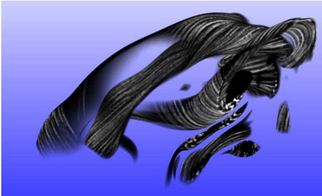
Figure 4.6: Two-field visualization, using enstrophy to define the opacity and the vorticity field represented by the LIC texture to define the color. The field lines of the vorticity field twist around the vortices, resulting in features reminiscent of "candy canes".
