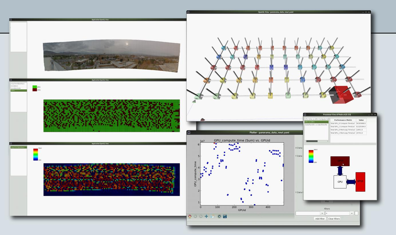
**Application View (top):** Final image generated by the application. **Application View (middle):** Image tiles, colored by if they were processed by CPUs or GPUs.
