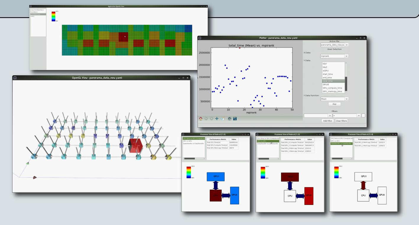
Application View: Data partitioning on the cluster and time taken by each node. A click on the partition automatically highlights the node in the other views.
