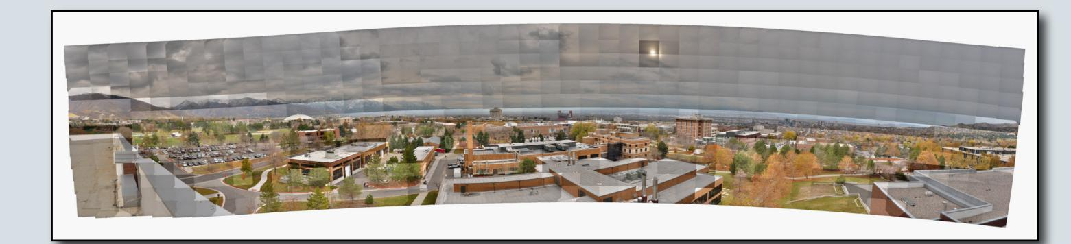
The algorithm decomposes the input images into 1024 X 1024 pixel sized tiles that are distributed across all MPI processes. Each of the MPI process then processes some tiles on a CPU or on the GPUs depending on available resources.
