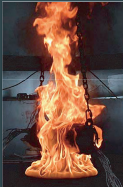
Above: Pool fire test facility. Below: Volume rendering of a JP8-surrogate fire produced by the integrated Arches/ICE simulation. This 1603 simulation ran on ALC for approximately 60 hours on 120 processors.
