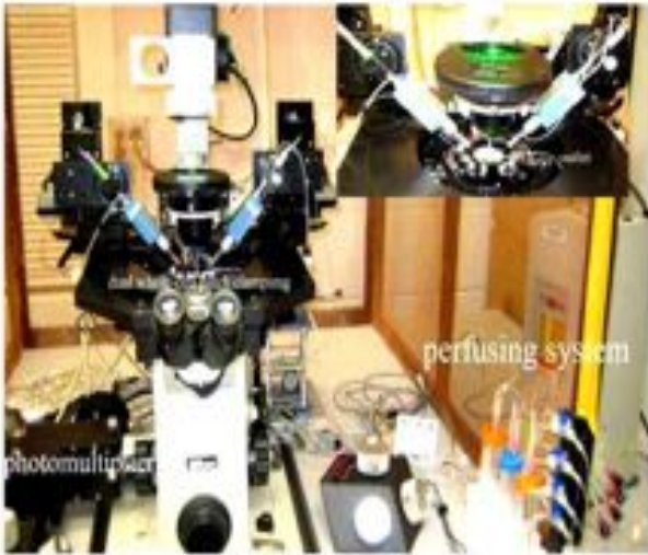
Figure 1. Double whole cell voltage clamp recording set up featuring the perfusion chamber and the photomultiplier required to detect pHi changes.
