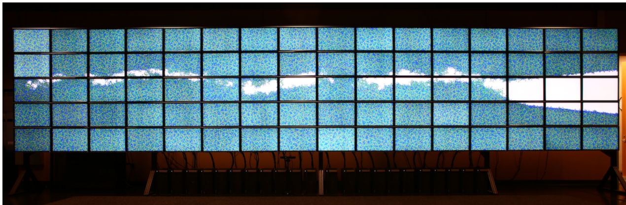
Figure 1: A 65536 \times 8192 (512 megapixel) frame buffer rendered on TACC Stampede using 128 Intel® Xeon Phi™’s and streaming at 2 fps to the TACC Stallion 328 megapixel tiled display.
