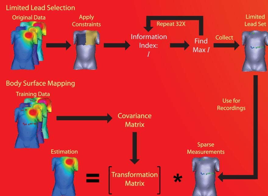
**Figure 1. Limited Lead Selection and Body Surface Mapping.** Body surface mapping is based on the statistical characteristics of a known set of torso potentials, specifically the covariance and standard deviation. With surface mapping, the full torso measurements can be taken using only 32 lead locations. The lead locations were chosen based on the information index obtained from the covariance and the standard deviation. For full explanation of the algorithm, refer to Lux, et al. [2]
