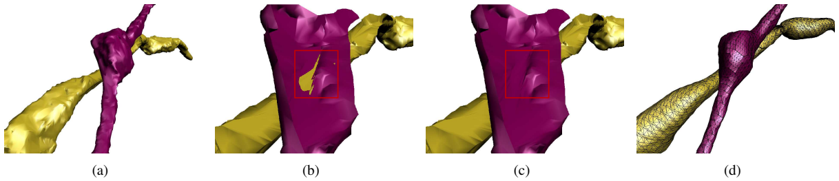
Figure 14: Results of running intersection removal on two axons that intersect. (a) Two axons whose reconstructions intersect between slices. (b) Zoomed in with part of the top axon cut away to reveal the intersection. (c) Result of intersection removal. (d) After smoothing.
