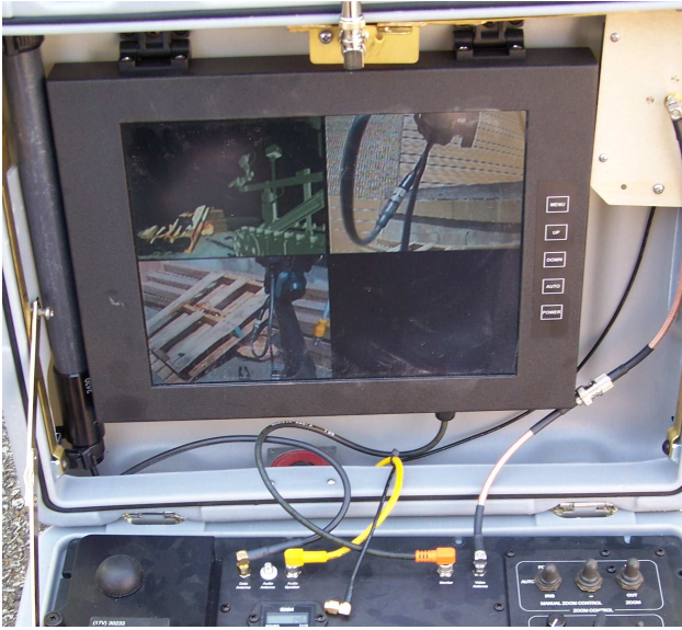
Figure 7: ASI's 3D visualization on a TALON OCU (upper left quad view). All processing is performed on the robot and the 3D model is displayed as a video stream that replaces a camera
