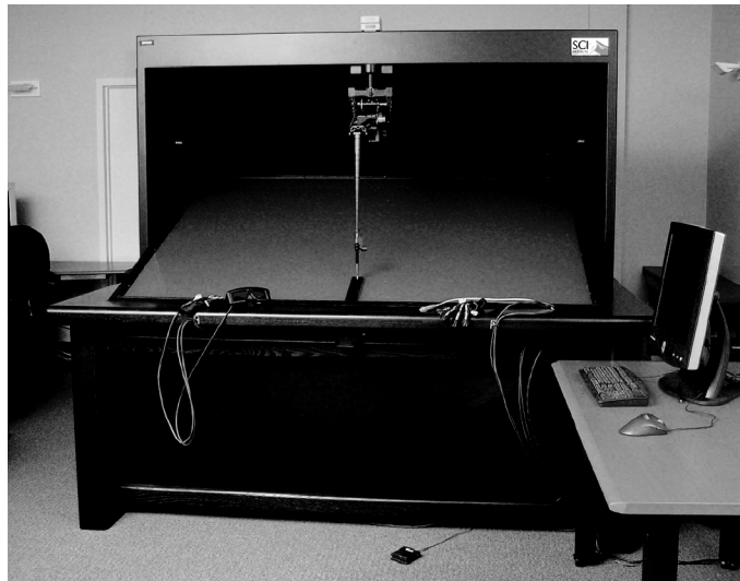
Figure 22.1 The Visual Haptic Workbench integrates a large workspace SensAble PHANToM with a Fakespace Immersive Workbench.
