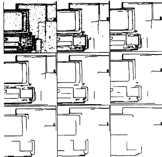
Fig. 16. Edges detected by thresholding the gradient in Fig. 14. Linking is not necessary. Thinning is only for the finer scales. Compare to Fig. 17 where thinning and linking have been used.
