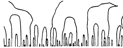
Fig. 2. Position of the edges (zeros of the Laplacian with respect to x ) through the linear scale space of Fig. 1 (adapted from Witkin [21]).
