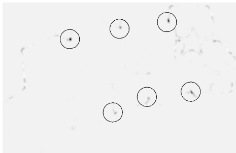
Figure 6.39 Detection of T-junctions in the image of the blocks with the detector \tau = \frac{\partial \kappa}{\partial w} L_w^6 . The same circles have been drawn as in figure 6.32.
