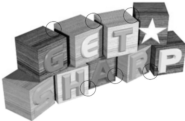
Figure 6.37 T-junctions often emerge at occlusion boundaries. The foreground edge is most likely to be the straight edge of the "T", with the occluded edge at some angle to it. The circles indicate some T-junctions in the image.
