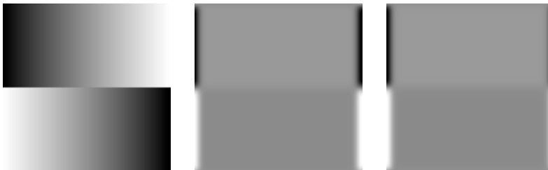
Figure 5.15 Boundary effects due to the periodicity of the Fourier domain.
