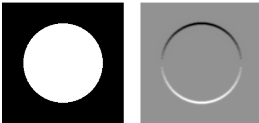
Figure 5.2 The derivative to y (right) at scale \sigma = 2 pixels on a 256^2 image of a circle (left).
