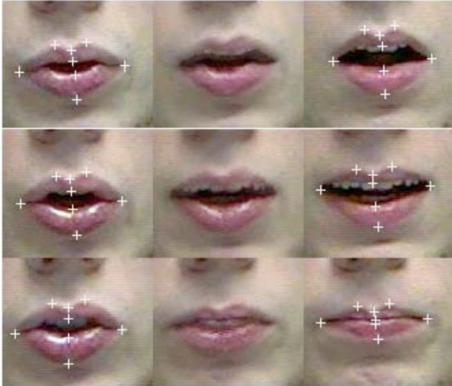
Figure 4. Synthesized viseme transitions. Central column contains transitional frames between the source and destination visemes.
