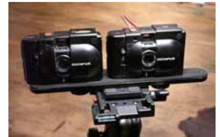
Parallel Cameras: Corresponding points on horizontal lines.
