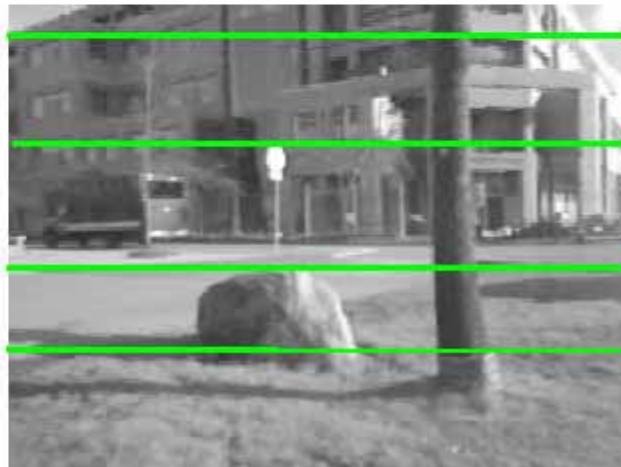
Parallel Cameras: Corresponding points on horizontal lines.
